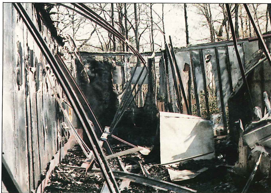
Looking out toward the rear of the strobe trailer. The dark panel at the left rear is the polyurethane crash pad determined as the point of origin.
